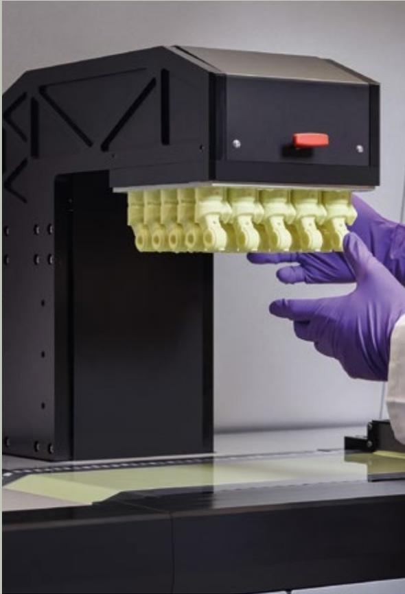
Featuring a large build volume and the unique capability of 3D printing both advanced ceramics and metals on one machine, optimized for high precision casting applications of silica shells and cores.
